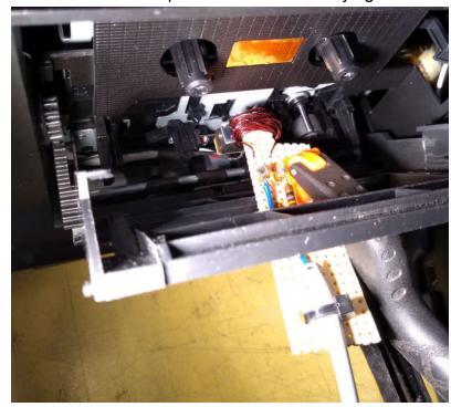
breadboard material. It's driven by an oscillator with a resistor in series to maintain constant current through the coil at all test frequencies. It's important to keep the coil in a fixed position while making measurements, hence the spring clamp you see in this photo. If you one a tape deck, I encourage you to make and experiment with a flux loop. You can learn a lot from it.
