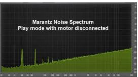
Well, we have an "AHA!" moment here. All of those mysterious noise spikes going well up the spectrum is coming from the motor. It's at a low enough level so that its inaudible on its own, but it contributes to the THD+N measurement, and provides plenty of frequencies to contribute intermodulation distortion to the tape playback.
