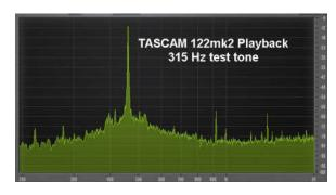
For comparison, here's a shot of the same tape played on my TASCAM 122mk2 deck, which measures substantially lower THD+N than the Marantz. This plot is zoomed in to show more detail where it matters. The overall noise of floor of the TASCAM is 10 dB lower than the Marantz, and only the 3<sup>rd</sup> and 5<sup>th</sup> harmonics of the
