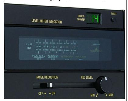
power indicator and is always on, leaving five steps of metering. When recording to tape, the last green segment, [-3 dB] is as high as you ever want to go. When the level reaches the first red segment, [0 dB], THD (total harmonic distortion) is greater than 10%. This isn't the "warm analog tape sound," rather, it's the "crappy cassette sound." Use the REC LEVEL control and pay attention to the level when recording on to a
