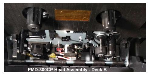
Note the erase head to the left on Deck B, and the lack of guides in the head area (of either transport).
