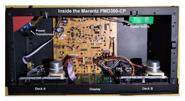
Decent quality Chinese-made components populate the cleanly laid out main circuit board. Circuitry is largely discrete (note the plethora of transistors) with a couple of dual op-amps and FET switching ICs.
