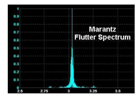
Notice the difference in the width of the spectrum spike and the height of the widened portion, which represent sidebands surrounding the test frequency created by speed fluctuations as the tape moves through the guides and across the heads.
