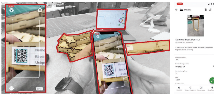
Figure 2. Interface of an early-stage material passport application, showing a QR code tagging prototype (left) and an experimental phone-based interface (right). Source: Grout, 2024.
