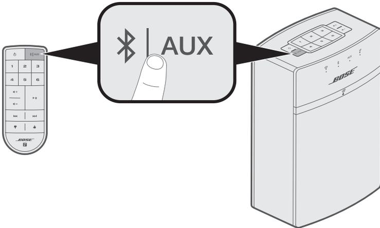
**Tip:** You can also press and hold
