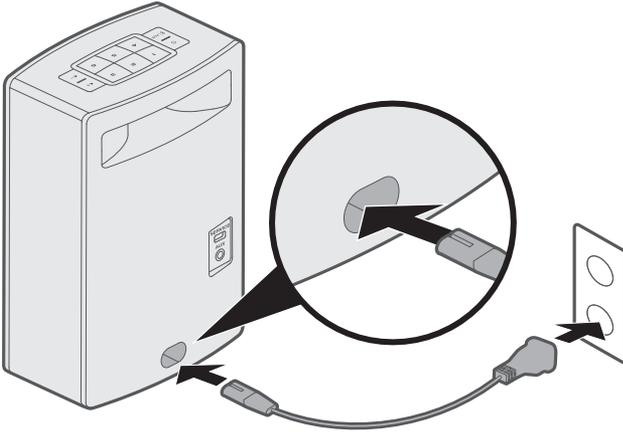
2. Plug the other end of the power cord into an AC (mains) power outlet.
